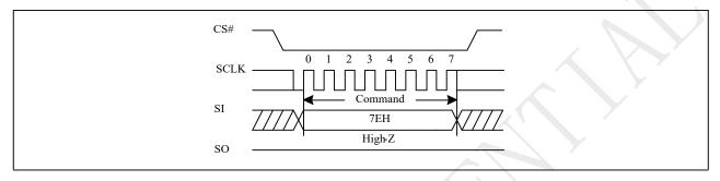
Figure 10-65a Global Block Lock (QPI)
