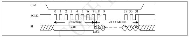
Figure 10-49a Erase Security Registers (ERSCUR) Sequence (QPI 44H)
