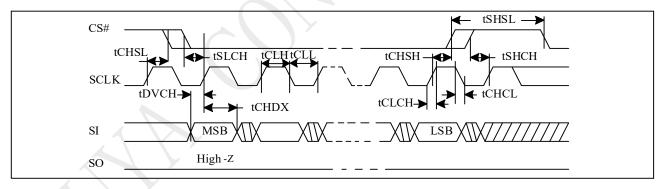
Figure 5-5 Output Timing
