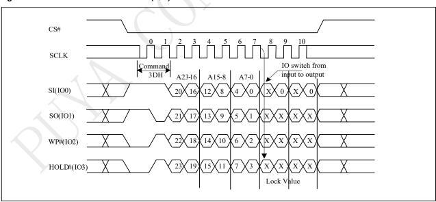
Note: 32-bit address is required when the device is operation in 4-byte address mode.
