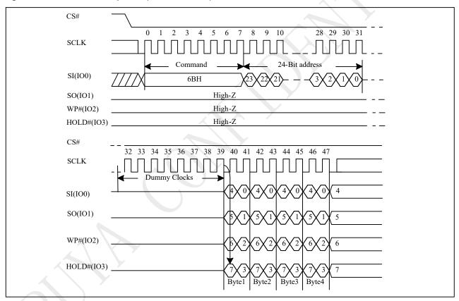
Figure 10-23 Quad Read Sequence (Command 6BH)
