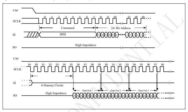
Note: 32-bit address is required when the device is operation in 4-byte address mode.
