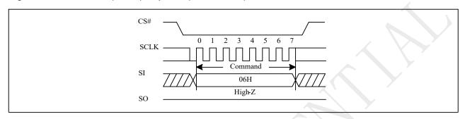
Figure 10-2a Write Enable (WREN) Sequence (QPI)
