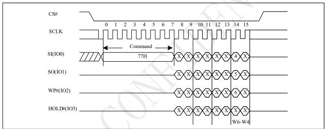
Note: 32-bit dummy bits are required when the device is operation in 4-byte address mode.
