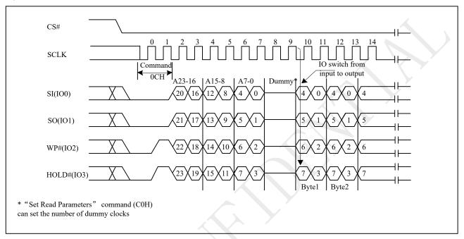
Note: 32-bit address is required when the device is operation in 4-byte address mode.
