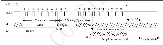
Figure 10-53a Read Electronic Signature (RES) Sequence (QPI)
