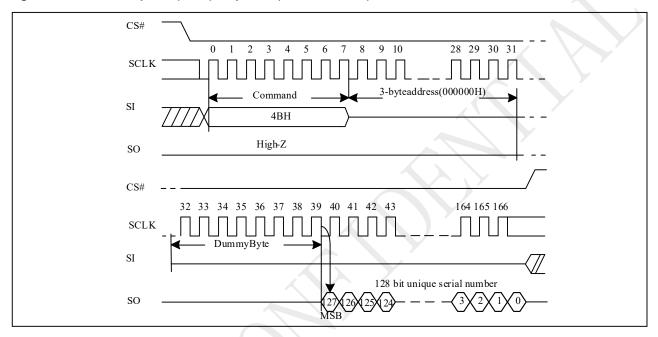
Note: 4 bytes address 0000\_0000H is required when the device is operation in 4-byte address mode.
