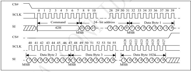
Figure 10-50a Program Security Registers (PRSCUR) Sequence (QPI 42H)
