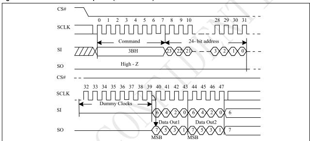
Figure 10-18 Dual Read Mode Sequence (Command 3B)
