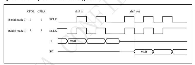
Figure 8-1 Serial Peripheral Interface Modes Supported
