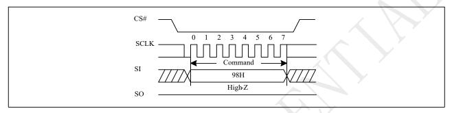
Figure 10-66a Global Block Unlock (QPI)
