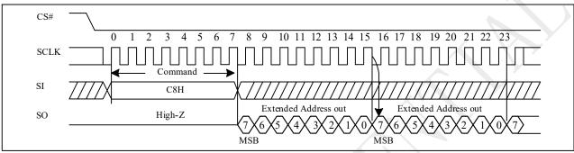
Figure 10-9a Read Extended Address Register Sequence (QPI)
