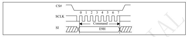
Figure 10-12a Exit 4-Byte Address Mode Sequence (QPI)
