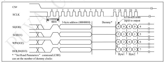
Note: 4 bytes address 0000\_0000H is required when the device is operation in 4-byte address mode.
