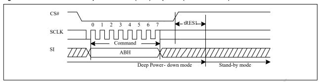
Figure 10-53c Release from Deep Power-down (RDP) Sequence (QPI)
