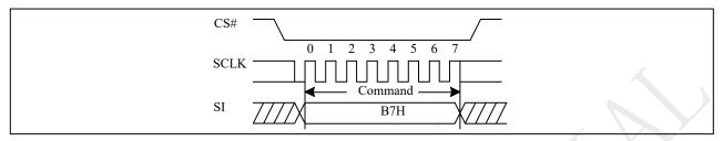
Figure 10-11a Enter 4-Byte Address Mode Sequence (QPI)
